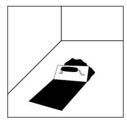
If the substrate cannot be made porous and will not have a topical moisture mitigation system installed, install a  $\geq$  6-mil thick polyethylene (PE) sheet, which is available at most home improvement stores. Use sheeting that is  $\leq$  10-ft. wide to prevent wrinkles and folds. Sheeting must be installed over the entire area and extend at least 2-in. up the walls. All seams must be overlapped and sealed according to the product instructions.
