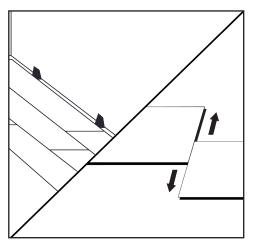
straightness tolerance is within 1/16-in. for lengths over 20-ft. or 1/32 in. for lengths under 20-ft. Complete the following rows starting with a cut piece, such as a piece from a previous row. Install the side joints before the end joints as instructed under "Side Joints" and "End Joints".
