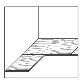
Note: plywood is a water-sensitive subfloor that may become damaged or deformed by topical liquids. To protect wood subfloors from topical water exposure, follow the Wet Area Guidelines.
