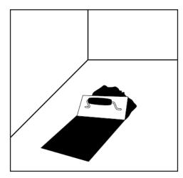
If the substrate cannot be made porous and will not have a topical moisture mitigation system installed, install  $a \ge 6$ -mil thick polyethylene (PE) sheet, which is available at most home improvement stores. Use sheeting that is  $\le 10$ -ft. wide to prevent wrinkles and folds. Sheeting must be installed over the entire area and extend at least 2-in. up the walls. All seams must be overlapped and sealed according to the product instructions.
