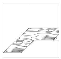
Note: plywood is a water-sensitive subfloor that may become damaged or deformed by topical liquids. To protect wood subfloors from topical water exposure, follow the Wet Area Guidelines.
